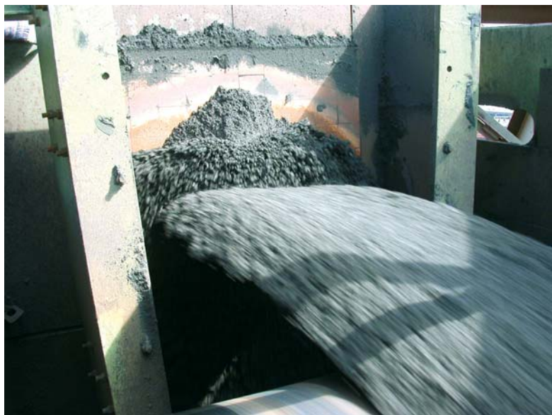
KERAFLEX-KRM used to fight abrasion and impact load in a discharge chute that handles coal and iron ore in a harbor loading and unloading plant
