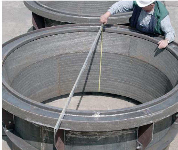
Cones of cement separators designed as self-supporting structures with plates made of KALMETALL-W 100 6+4 hard overlay welding; their diameter is 3 000 mm
