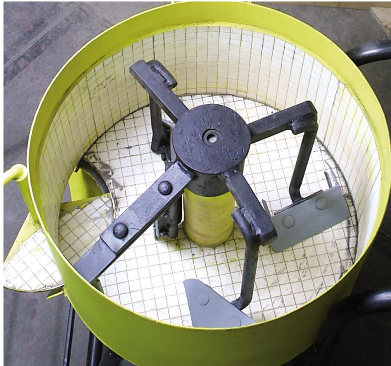
Wear protected forced-circulation mixer for bulk construction materials. High alumina ceramic mosaics are well adaptable to the specific geometry.
