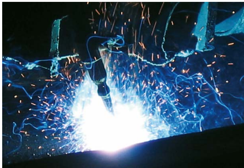
Hard-facing of plant components with flux cored wires or stick electrodes
