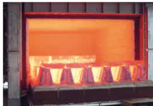
Heat treatment at 1,200 °C / 2,192 °F
