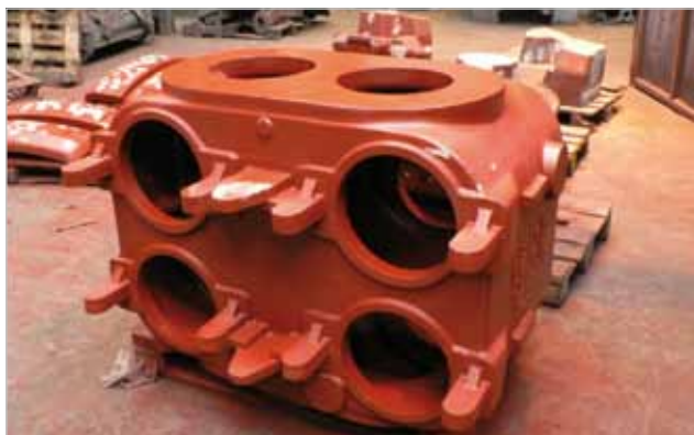
Housing for an air-conditioning unit
