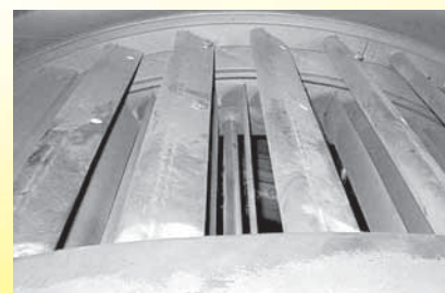
Guide vanes of a separator made of KALSICA-A operated in combination with a coal pulverizer
