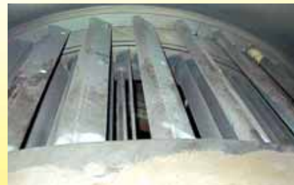
Guide vanes of a separator operated in combination with a coal pulverizer
