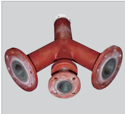
Pipe branch made of KALSICA-S for handling granulated blast-furnace slag: inside diameter 80 and 100 mm, 10 mm wall thickness, high abrasive wear, impact wear due to turbulence, 400 °C / 752 °F, little wall thickness
