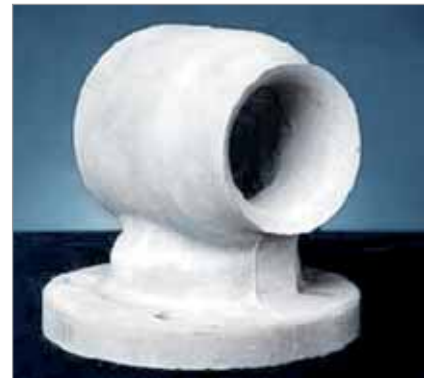
Lime slurry nozzle made of KALSICA-N in a flue-gas desulphurization plant: inside diameter 80 mm, high abrasive wear, 80 °C / 176 °F, manufactured in one piece as a self-supporting structure
