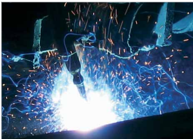
Hard-facing of plant components with flux cored wires or stick electrodes
