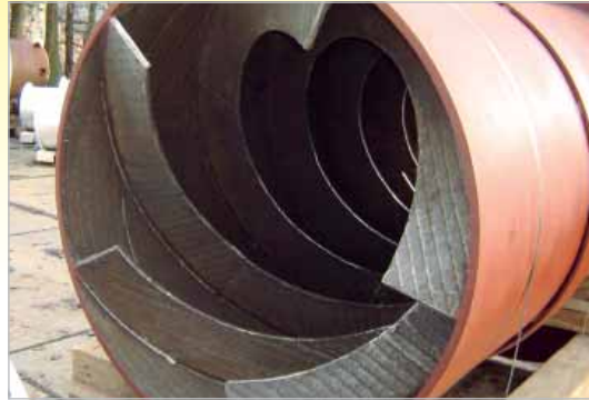
Screw conveyor lined with KALMETALL-W
