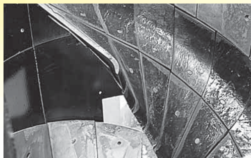
Shaft spiral used for hard coal mining and fitted with time-tested KALMETALL-C lining
