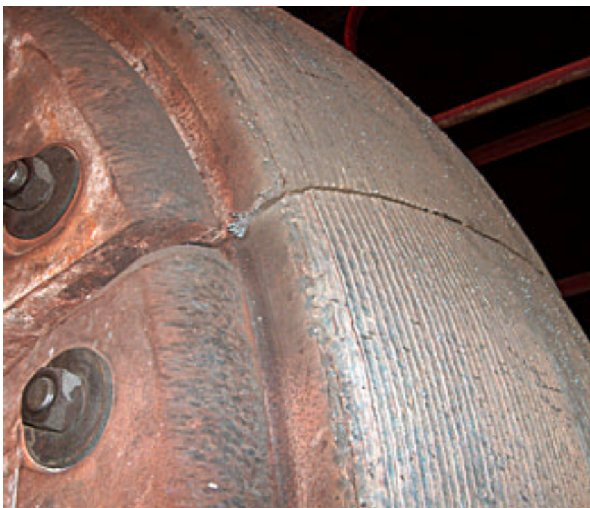
Fig. 13: For large diameters grinding roller outer wear sections may be of segmented type; this illustration shows a regenerated design
