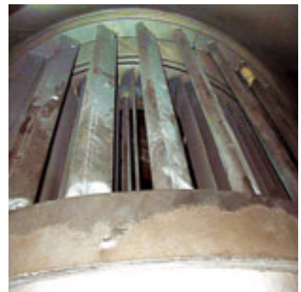
Fig 8: Guide vanes of a separator in a vertical mill for coal made of KALSICA-A silicon carbide ceramics
