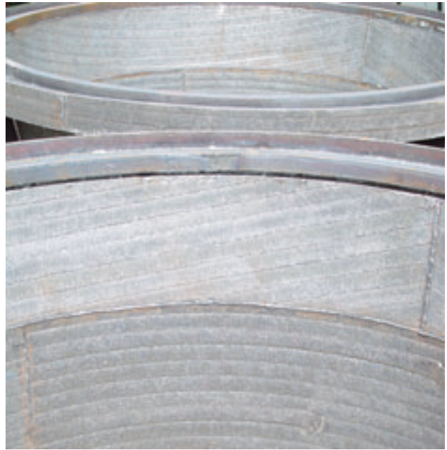
Fig. 7: Separating cones of classifiers can be efficiently protected with KALMETALL-W 100 6+4 hard overlay welding; the illustration shows a self-supporting structure of 3,000 mm diameter
