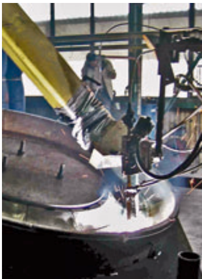
Fig. 17: Regeneration of a worn grinding table in the special Kalenborn shop
