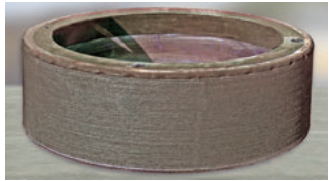
Fig. 16: Regenerated grinding roller with a rectangular cross section using KALMETALL-W 100 hard overlay welding; the diameter is 1,500 mm
