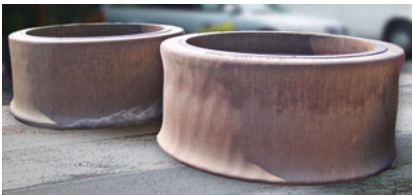
Fig. 1: Grinding rollers in roller mills are subject to considerable wear; here worn down raw meal grinding rollers prior to regeneration
