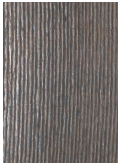
Abb.19: Knowledge gained during the regeneration of grinding elements ensure excellent quality and durability of the overlay welding; in addition, the weld pattern shown enhances the material feed between the grinding elements
