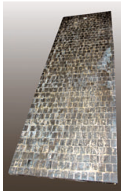
Fig. 3: Wear plates are armored with soldered-on hard metal tiles in cases of extreme wear and extreme impact
