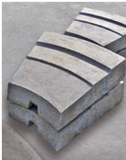
Fig. 12: Grinding table segments of a 5,000 mm diameter roller mill made of KALMETALL-C; smaller diameters are cast in one piece
