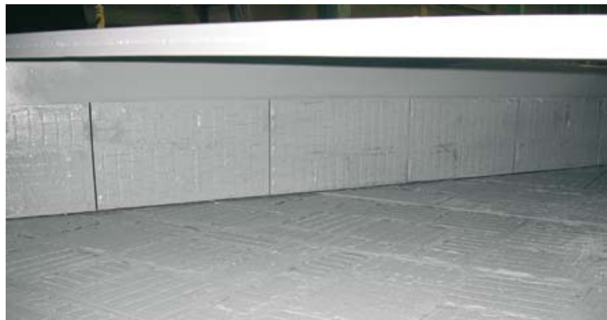
Custom-fit mounting of KERAFLEX-WRM elements in a chute: their maximum size is 500 x 500 mm; the elements can be individually matched to the specific requirements
