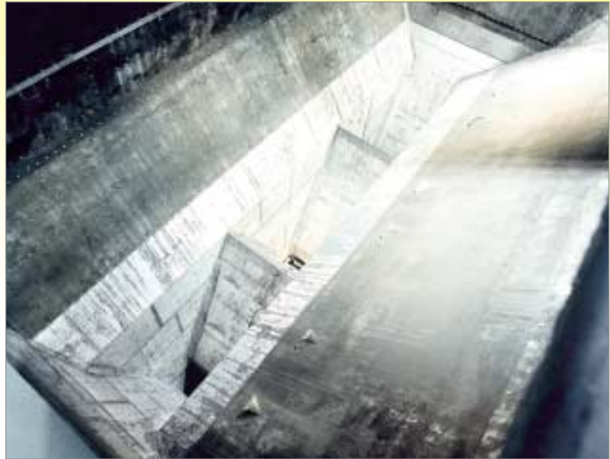
Slide promoting lining combination in the lower part of a high-level storage bin: fitted with KALEN linings on the inclined surfaces and KALINOX within the outlets which are subject to more intense wear.
