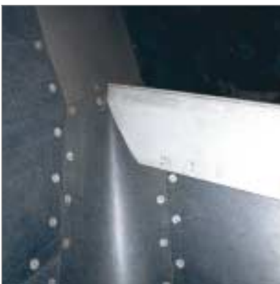
KALINOX angles protect the saddle of the bin lined with KALEN.
