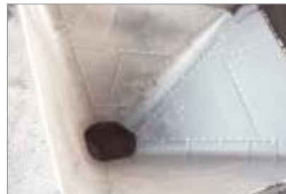
Bunker for fine coal: The slide promoting lining ensures the material flow without sticking and clogging.
